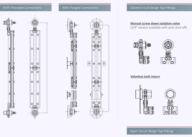
(TOP OF GAUGE MUST BE MIN. 100mm ABOVE TANK TOP)
