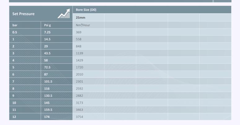
Capacity Table - In accordance with ASME BPVC.XIII, AIR at 60°F and 14.7 psia/scfm. SCFM Type 106/116: Flow rates at 10% above the set pressure.
