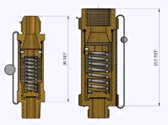
Maximum permissible built up back pressure = 10% of set pressure at or below which flow is not reduced. Stable operation on flows down to 50% of valve rated capacity.
