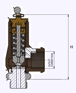
Maximum permissible built up back pressure = 10% of set pressure at or below which flow is not reduced.
