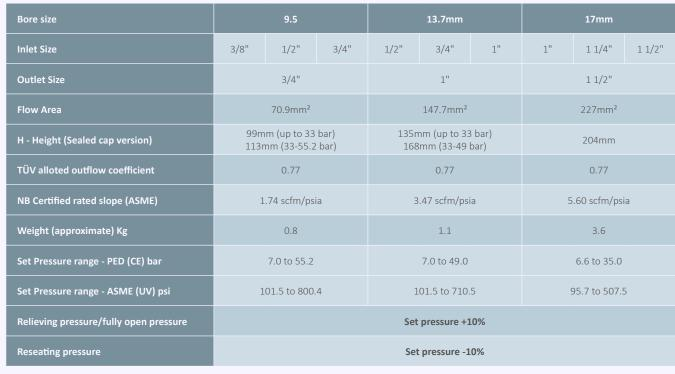
Maximum permissible built up back pressure = 10% of set pressure at or below which flow is not reduced. Stable operation on flows down to 50% of valve rated capacity.
